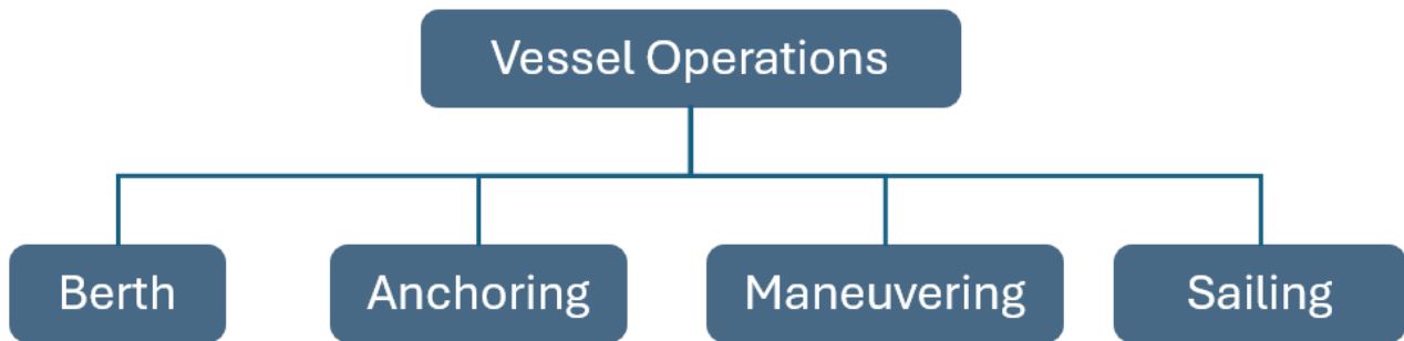
Figure 16: Vessel operations while within port basins. Each operation requires different usage of the main and auxiliary engines (see Table 1 ).
